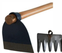
Spade & Concrete Panja
